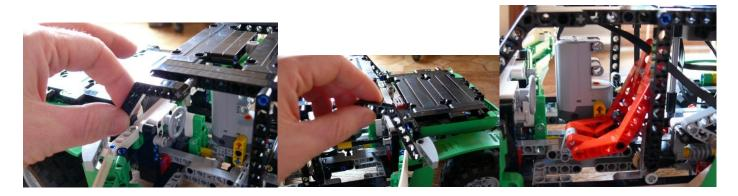
Plug the receiver cable on the battery box, and insert the box into the car. Add a pin to lock the battery box in place.
