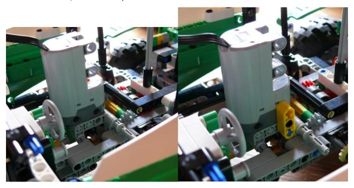
Return the model. Align the front wheels and push the axle thru the knob wheel so it plugs into the servomotor. I used a screwdriver to do this because my fingers are to big.
